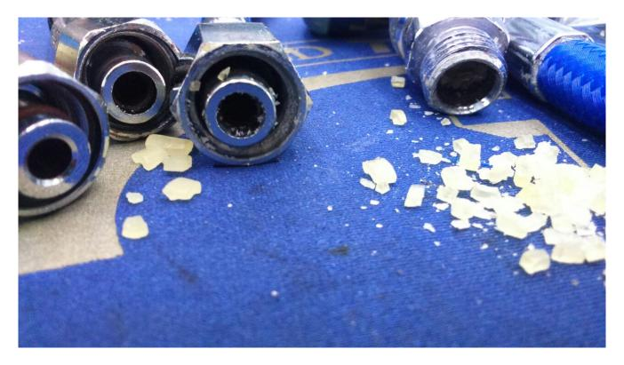
It is hard to predict the time required for a polyester-TPU liner to decay, but available information suggests that at 30°C and high humidity, exposed hoses could decay in less.
