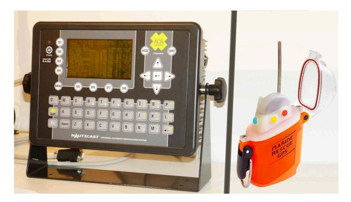
An **AIS - MOB**-system works in a different way to a PLB. Without going into detail, the system is designed to be carried by ship crew members and used in the event of a man overboard situation. When activated, this system transmits a MOB message containing the person's position and identification ID via an AIS. The transmission will be detected by all AIS equipped vessels within range. An inbuilt GPS receiver and strobe helps rescuers pinpoint your precise location in the water.
