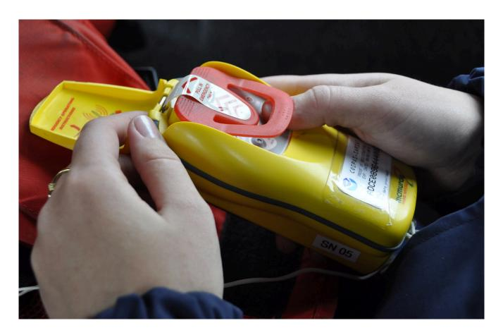
A **PLB** is a personal locator beacon, allowing SAR Services to locate a person on land or sea. When activated, the PLB will transmit a coded message on the 406 MHz distress frequency, which is monitored by the COSPAS-SARSAT<sup>2</sup> satellite network. This message is then forwarded via an earth station to the nearest Rescue Coordination Centre (RCC), which will activate the local SAR services.
