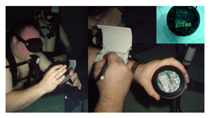
During the test, the diver looks straight into the LED at a comfortable distance. The investigator then increases or decreases the flicker frequency by rotating the ring. When the diver sees the LED change from flicker to fusion, or vice versa, the test is stopped, and the fusion frequency is recorded.
