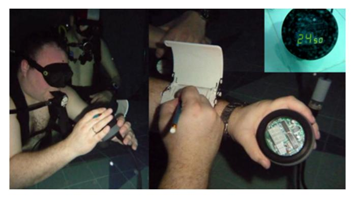
During the test, the diver looks straight into the LED at a comfortable distance. The investigator then increases or decreases the flicker frequency by rotating the ring. When the diver sees the LED change from flicker to fusion, or vice versa, the test is stopped, and the fusion frequency is recorded.
